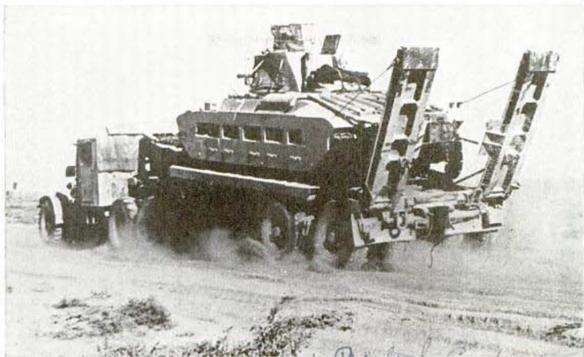
Two oblique tracks at back of trailer form ramp on which disabled tank is loaded and unloaded
